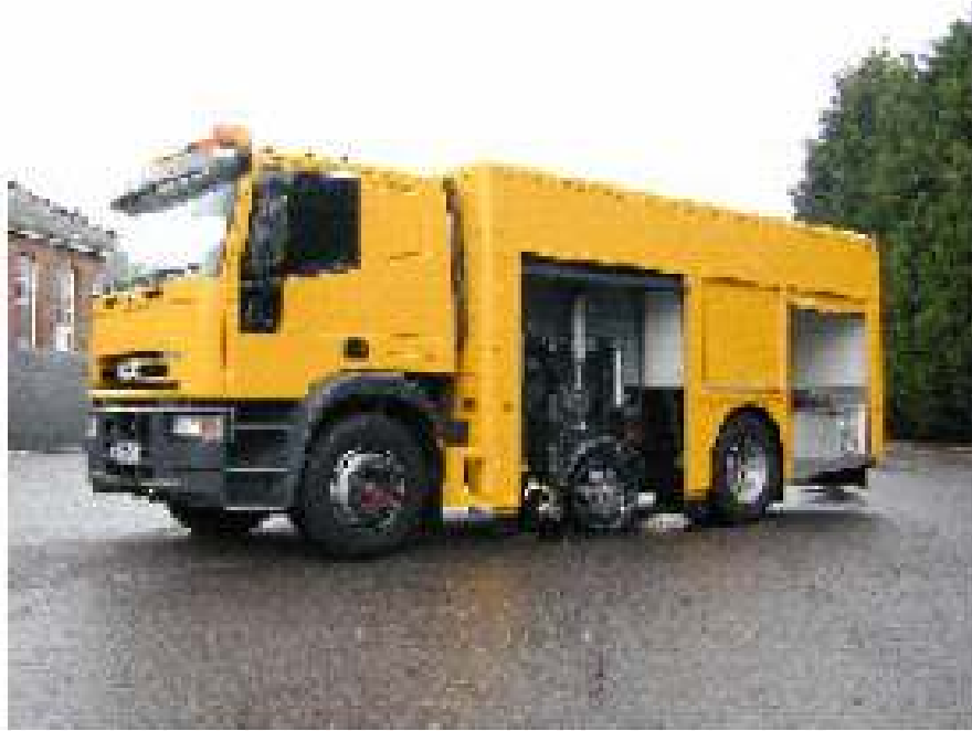
The SCRIM machine used for skid resistance surveys
