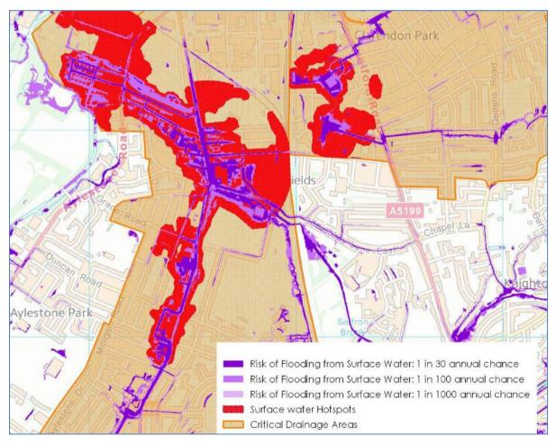
Figure 4.13 Example of surface water flood risk mapping.
